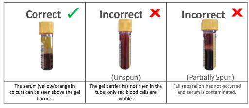
Tubes must be centrifuged at a minimum speed of 1500-2000g. Please check that your centrifuge is set to achieve an rpm to generate the required relative centrifugal force ("g"). Instructions are provided on the following page alongside a conversion chart to determine the correct rpm setting for your centrifuge.
